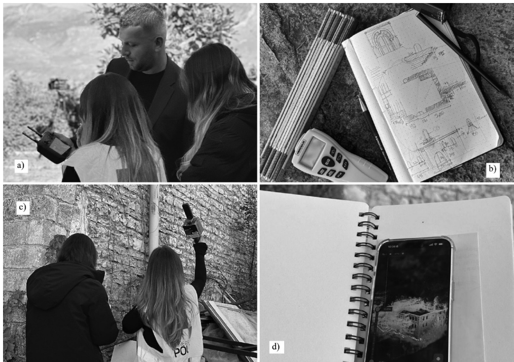
Fig. 2. Integrated on-site data acquisition procedures for the digital survey of the Topulli House: a) UAV-based photogrammetry using DJI Mavic 3E for contextual 3D modeling and orthophotos; b) Manual sketches and metric measurements to validate non-digital data; c) Terrestrial LiDAR scanning with FJD Trion P1 for high-precision façade geometry; d) Real-time point-cloud monitoring within the FJD platform for in-situ data validation.
