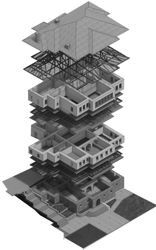
Fig. 6. 3D Axonometric exploded view of the building developed in a BIM environment using Autodesk Revit, with post-processing enhancements and graphical refinements carried out in Adobe Photoshop to highlight architectural stratification and element assembly
