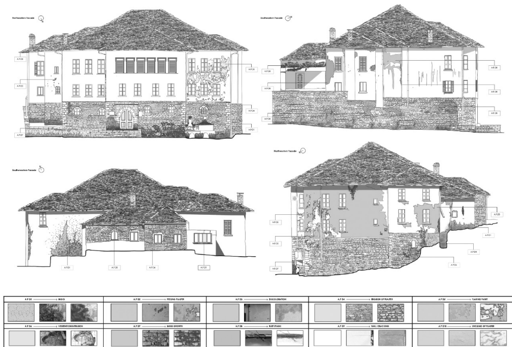
Fig. 4. Current pathological analysis conducted on the façades of the Topulli House, identifying material deterioration, structural anomalies, and signs of environmental damage
